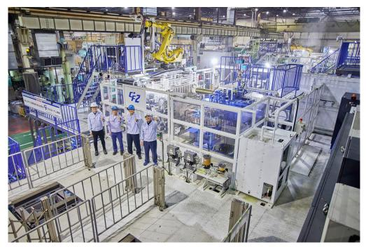
High-temperature processes like casting and painting present significant hurdles in achieving fossil-free production. The new die-casting machines installed at the Iwata Main Factory cut CO<sub>2</sub> emissions by 49% compared to the previous machines.
